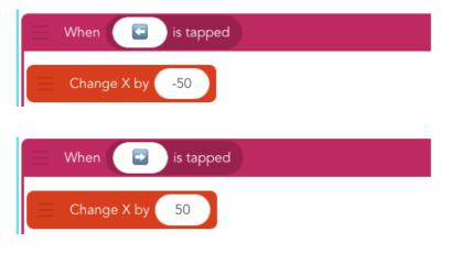
Moving left is changing the X position by a negative amount, and moving right is changing the X position by a positive amount.
